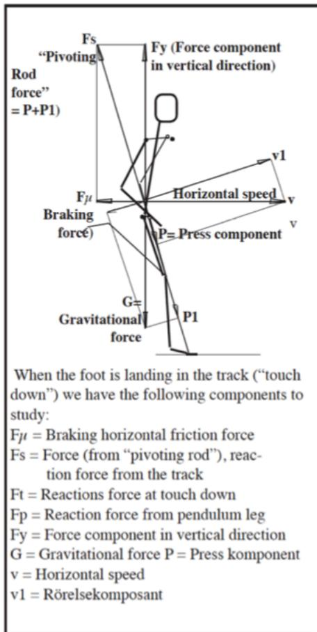
Fig 30a shows emergence of the brake power ( $F_{\mu}$ ).
